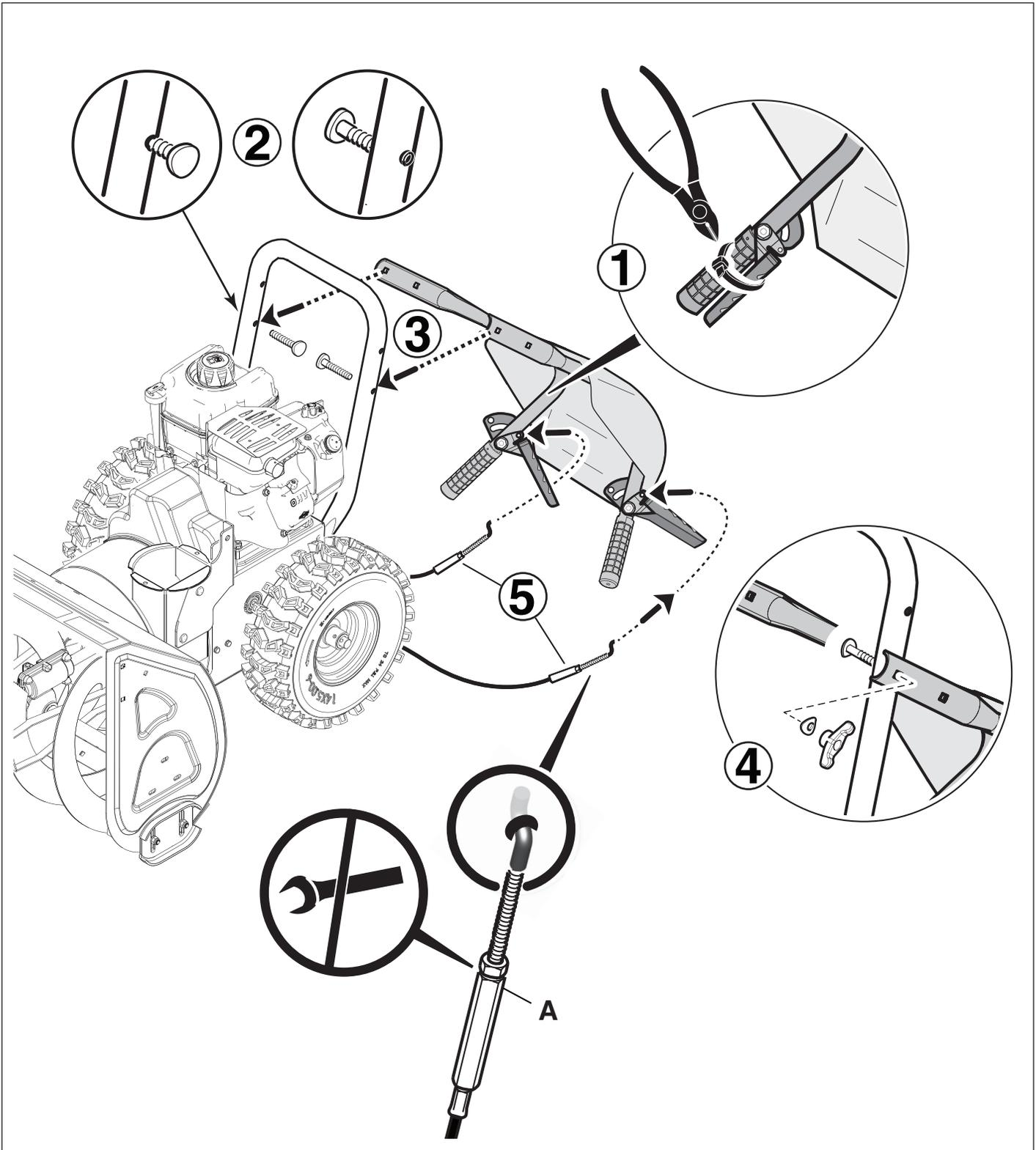
**en** Check tension on both cables **8** . Cables should deflect slightly with moderate finger pressure. If an adjustment is needed, see the Operator's Manual.
