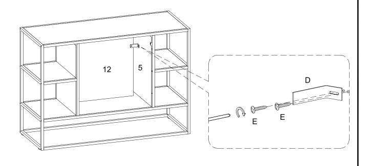
Attach bracket (D) to part (5) using screw (E) with screwdriver.
