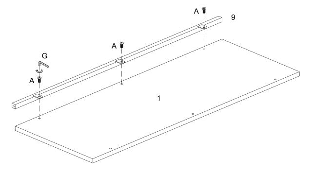
Attach part (9) to part (1) using bolt (A) and Hex Key (G).
