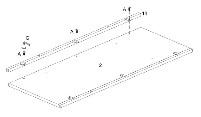
Attach part (14) to part (2) using bolt (A) and Hex Key (G).
