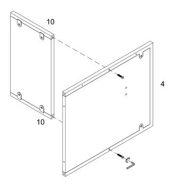
Attach part (4) to part (10) using bolt (C) and Hex Key (G).
