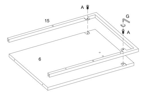
Attach part (15) to part (6) using bolt (A) and Hex Key (G).
