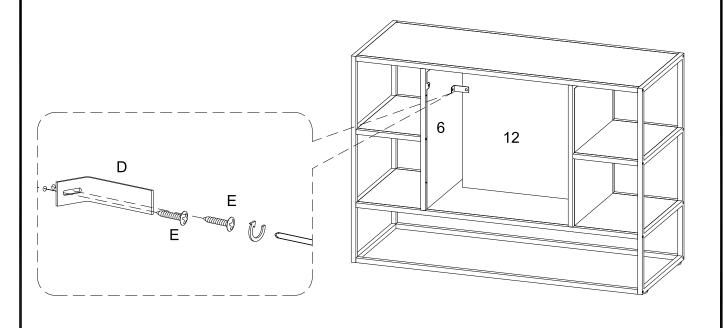
Attach bracket (D) to part (6) using screw (E) with screwdriver.
