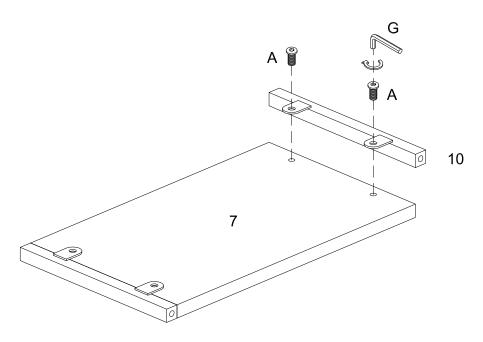
Attach part (10) to part (7) using bolt (A) and Hex Key (G). Repeat this step.
