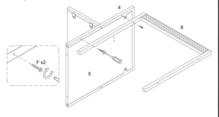
Attach part (8) to part (4) using screw (F) and screwdriver.
