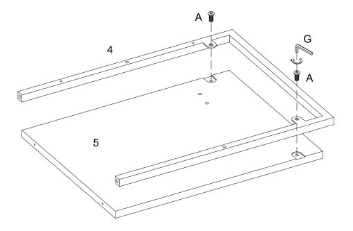
Attach part (4) to part (5) using bolt (A) and Hex Key (G).
