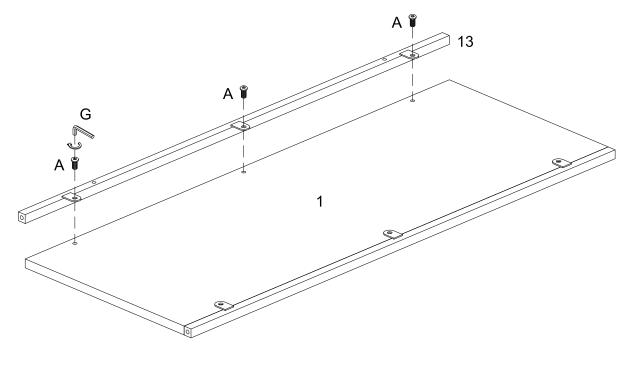
Attach part (13) to part (1) using bolt (A) and Hex Key (G).
