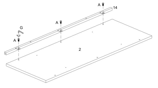
Attach part (14) to part (2) using bolt (A) and Hex Key (G).
