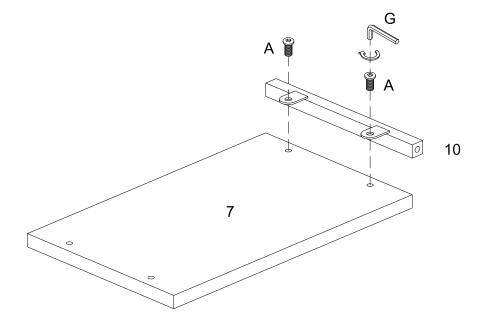
Attach part (10) to part (7) using bolt (A) and Hex Key (G). Repeat this step.
