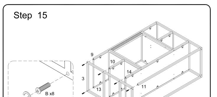
Attach part (3) to part (9,10,11,13,14) using bolt (B) and Hex Key (G).
