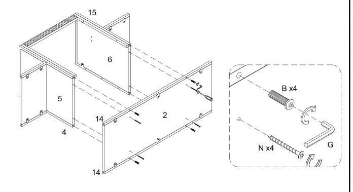
Attach part (2) to part (4,5,6,15) using screw (N) with screwdriver, and bolt (B) with hex key (G).
