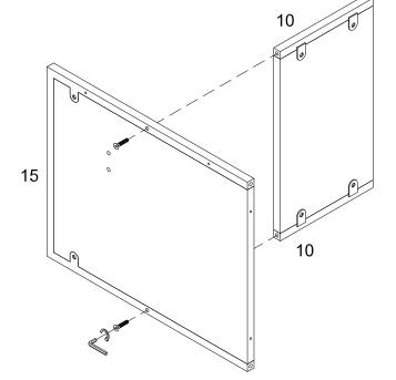
Attach part (15) to part (10) using bolt (C) and Hex Key (G).
