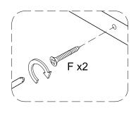
Attach part (8) to part (15) using screw (F) and screwdriver.
