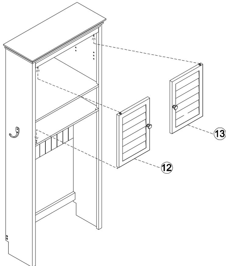
**Step 9.** Drill two 11/32" holes where you want to secure your pantry .The hole should be at the same height as the hole in the back panel (Part #8) of this unit . Tap Wall Anchor(J) into the hole . Insert Screw (K) through Back Panel (8) into Wall Anchor (J).
