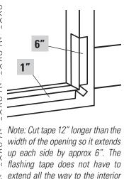
**STEP 1.** Check to be sure that the rough wall opening is square (diagonals measure the same). Cut a piece of flashing tape 12" longer than the opening width. Apply tape at the bottom of the opening so that it overhangs 1" to the exterior and 6" up each side of the opening, as shown.
