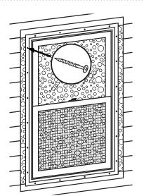
**STEP 3**. Once the unit is square in the opening, secure the window by using #8 x 2" galvanized or stainless steel pan head screws placed through the installation flange.
