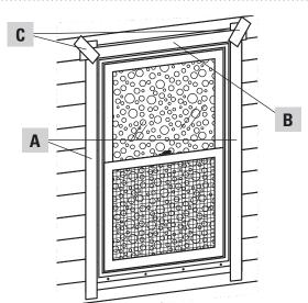
**STEP 4**. Apply flashing tape to sides first, then across the top and lastly to the upper corners. (**A**) Cut two pieces of tape 4" longer than the frame height of the window. (**B**) Cut one piece of flashing tape long enough to go across the top of the window extending at least 1" past the side flashing tape on both sides. (**C**) Apply tape to the top two corners of the window extending at least 1" past the corner tape seams. *DO NOT SEAL ACROSS THE BOTTOM INSTALLATION FLANGE.*
