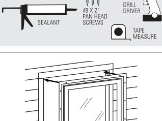
**STEP 2.** Place the window into the center of the opening, making sure that the window is level and centered within the rough opening. Apply sealant to the exterior of the buck frame then place the window into the center of the opening. Make sure that the window remains centered within the rough opening.
