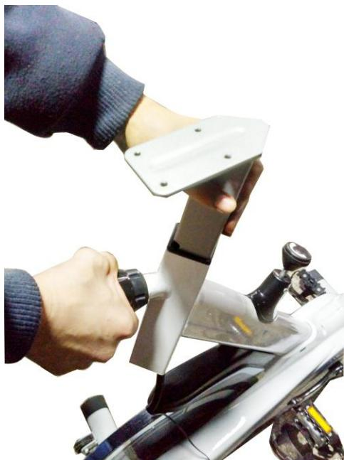
4、Take out the handle and then put four holes of handle into screwed hole, next put washer and through Cylinder head screw, then support by screws one by one.
