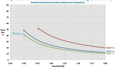
Temperature Rise versus Flow Rate @ 208 V
