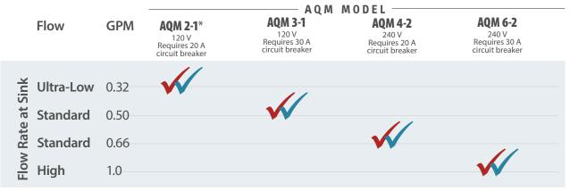
\*AQM 2-1 is internally restricted to 0.32 GPM.
