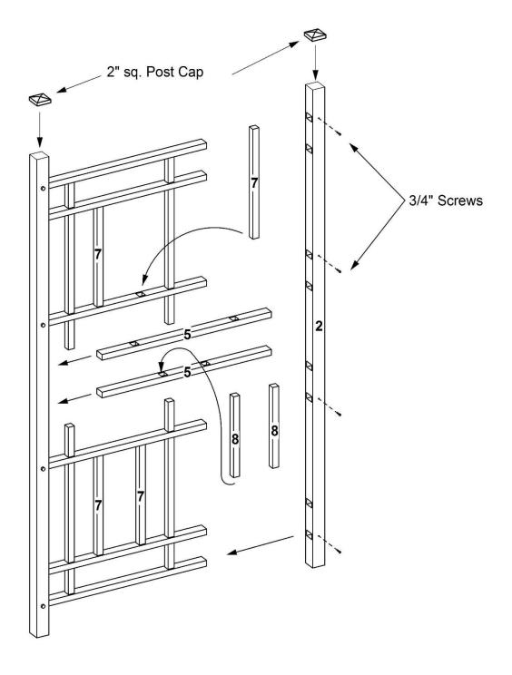
Insert two 27½" middle cross rails (part 5) into remaining routed holes in side of post, inserting free ends of 26½" vertical rails into middle cross rail. Insert four 16¾" vertical rails (part 7) into remaining holes in inside cross rails. Insert two 13" vertical rails (part 8) into remaining holes in middle cross rails. Insert free ends of cross rails into 74" right post (part 2).
