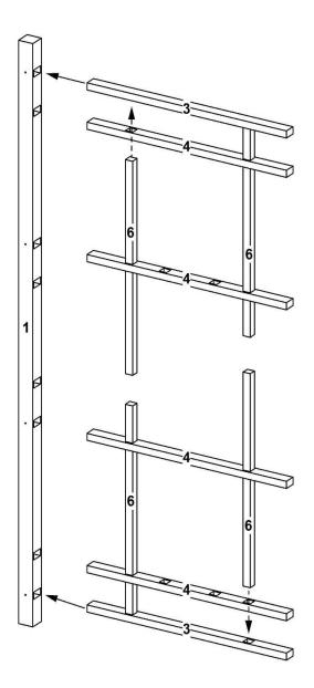
Starting at bottom of 74" left post (part 1), insert one 27½" outer cross rail (part 3) and two 27½" inner cross rails (part 4). When inserting two inner cross rails insert sides with four routed holes facing each other. Insert two 26½" vertical rails (part 6) through outer holes of inner cross rails and into outer holes of outer cross rail.
