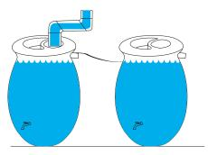
During the winter months you should drain the water inside the Castilla Rain Barrel and leave the valve in the hose in the open position. You may want to bring your Rain Barrel inside to protect it from the elements, but this is not necessary. The unique design of the Castilla Rain Barrel allows it to withstand extreme weather.
