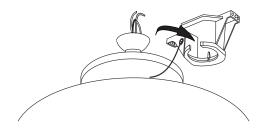
Lift fan assembly onto mounting bracket.
