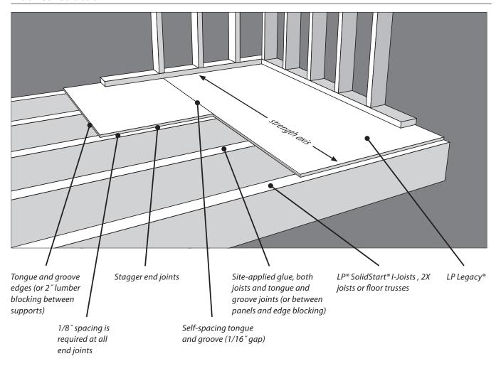
**Note:** Provide adequate ventilation and use ground cover vapor retarder in crawl space. Panels must be dry before applying finish flooring.
