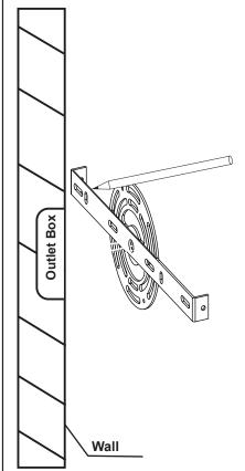
Raise mounting bracket (A) to the wall. Mark location for the plastic anchors (B). Drill holes for plastic anchors (B). Insert plastic anchors (B) into hole.
