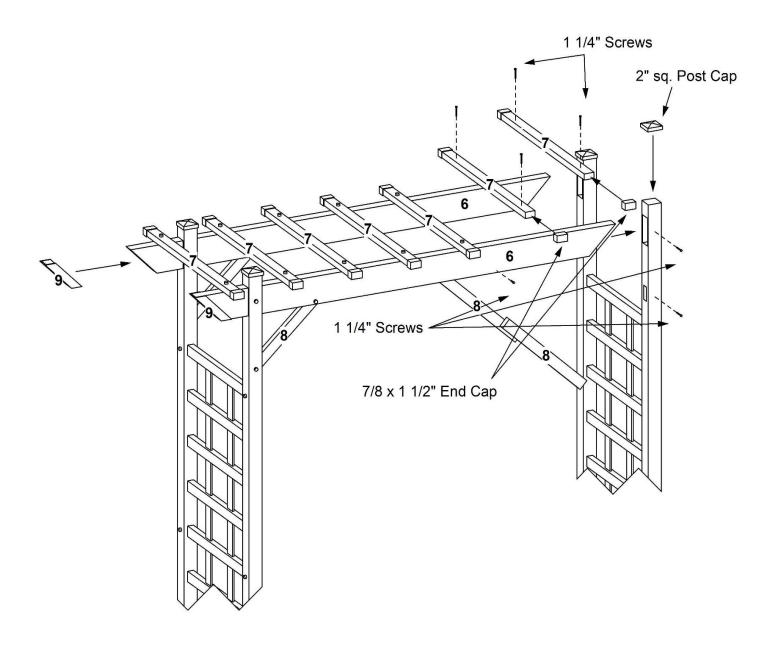
Insert two 16" corner braces (part 8) into each 64" arbor top (part 6). Slide ends of arbor top rail through holes at top of post, inserting corner braces into posts. Measure 9 inches from tips of arbor top rails and slide posts so outside of post in 9 inches from end of arbor top rails. Using three 1¼" screws per post, fasten together posts, arbor top rails and corner braces.
