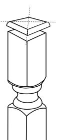
**Step 2:** Use power drill with a 1/4" drill bit to predrill a hole at the center mark on the treated deck post.
