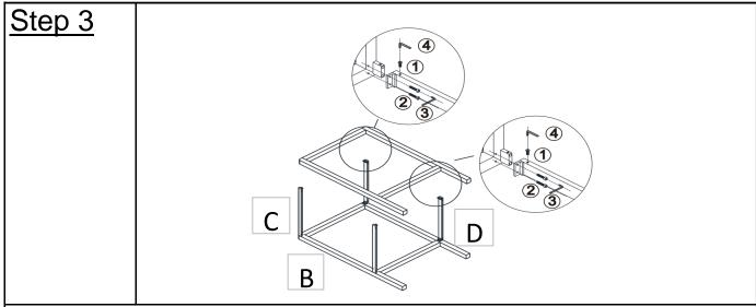
Attach Leg(B) to Top Side Bars(C) and Footrests(D) using Bolts(2) with Allen Key(3) as shown above.
