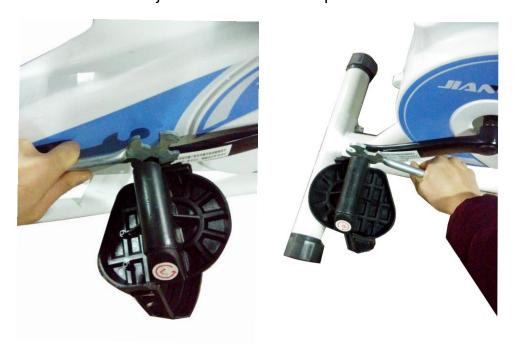
2). The feet straps are marked with L and R. Please drop 2 red screw locking liquid in R
