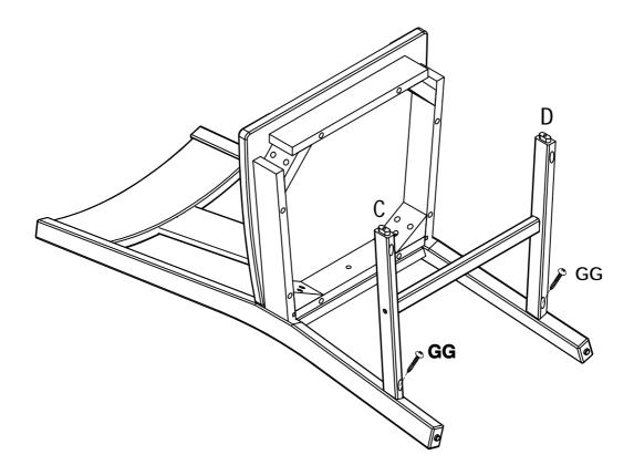
**5** Use screw(GG) to fasten left leg(F) and right leg(G) to side rails(C&D)
