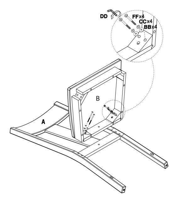
2 Use allen key (DD) to drive the screw(AA) with washers(CC&BB) as shown
