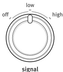
Turn the SIGNAL knob to select the desired setting (Off, Low, or High). The Signal produces an audible sound when the drying cycle is finished. Promptly removing clothes at the end of the cycle reduces wrinkling.
