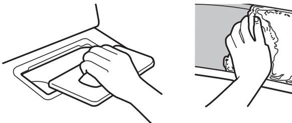
Clean the lint screen before each load. Pull the lint screen out of its holder. Roll lint off the screen with your fingers. Do not rinse or wash screen to remove lint. Push the lint screen firmly back into place.
