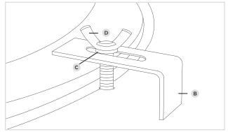
STEP 6 - ATTACH UNDERMOUNT CLIPS
