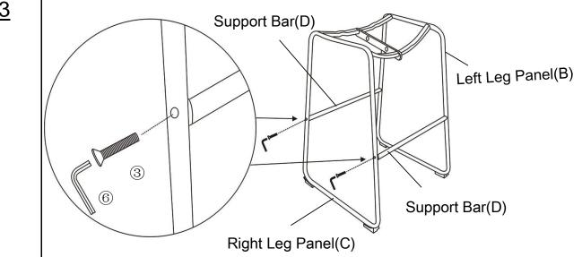
Then place Support Bars(D) between Right Leg Panel(C) and Left Leg Panel(B) as shown in picture above.
