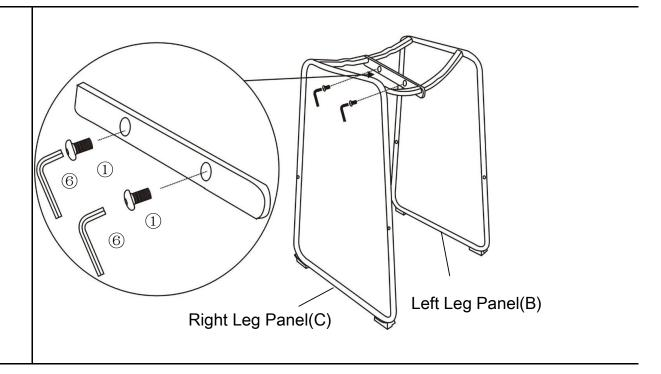
Align Left Leg Panel(B) with Right Leg Panel(C) as shown in the picture. Attach Left Leg Panel(B) to Right Leg Panel(C) using Short Bolts(1) with Allen Key(6).
