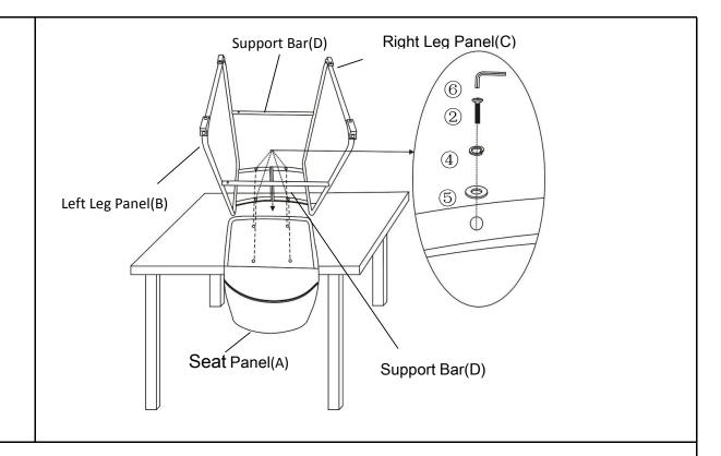
With the help from your partner, place the Seat Panel(A) facedown. Align the Left Leg Panel(B) and Right Leg Panel(C) with Seat Panel(A). Attach using Middle Bolts(2), Spring Washers(4), and Washers(5) with Allen Key(6).
