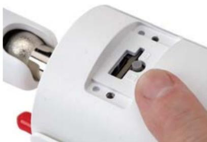
**NOTE:** SD memory card slot and reset button can both be accessed by removing the bottom panel from the camera with a standard screwdriver. Reattach panel before mounting cameras.
