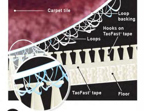
The concept is based on a hook and loop fastening system using carpet tile which has a loop material covering its entire underside. Hook tapes are fastened to the sub-floor by means of a pressure-sensitive adhesive. The hook and loops 'engage' and form a mechanical bond, which holds the carpet in place.
