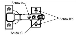
**SIDE TO SIDE ADJUSTMENT:** Door is adjusted side to side by turning **"Screw A"** clockwise or counterclockwise.
