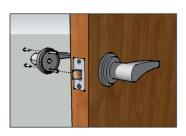
Secure with bolt through fixings.
