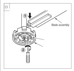
Install blade assembly with screws provided, aligning each of the holes as shown and tighten all screws securely. Repeat this process for remaining blades.
