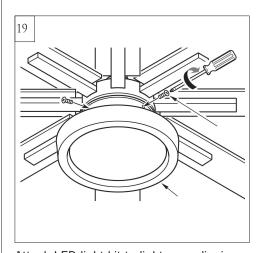
Attach LED light kit to light pan, aligning the holes on LED light kit with the holes on light pan. Reinstall the set screws removed in step 17. Tighten screws securely.
