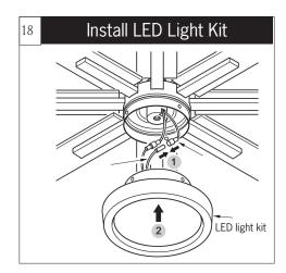
Connect white wire from fan to white wire from LED light kit and then connect blue (or black) wire from fan to blue (or black) wire from LED light kit.
