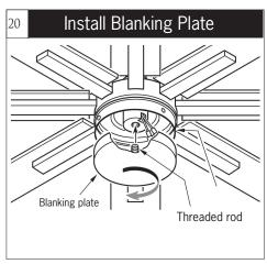
Align the threaded rod in blanking plate with the screw hole in light pan and Install it by turning clockwise till tight.
