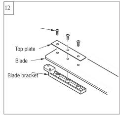
Align the holes of blade bracket, blade and the top plate of blade bracket. Install blade bracket with blade and top plate by 3 blade screws provided. Tighten screws securely. Repeat this process for remaining blades.
