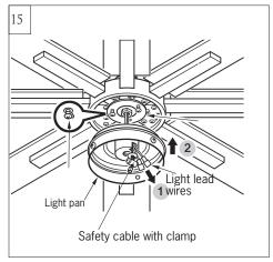
Lift light pan up, thread the light lead wires and the safety cable with clamp through the slot in light pan as shown.
