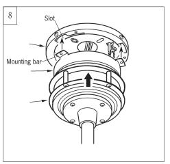
Lift motor assembly, aligning the mounting bar with the slots on mounting plate, and twist clockwise till lock.
