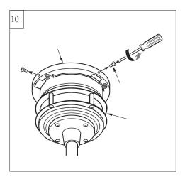
Remove set screws from mounting plate. Keep screws.
