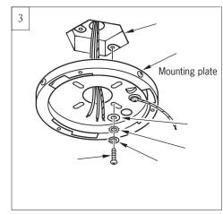
Use metal outlet box suitable for fan support and use only the screws provided with the outlet box (must support 35 lbs). Before attaching fan to outlet box, ensure the outlet box is securely fastened by at least two points to a structural ceiling member (a loose box will cause the fan to wobble). Remove the two outlet box screws provided with the box, aligning the holes of the mounting plate with the holes of the outlet box. Reinstall the 2 outlet box screws securely.
