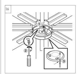
Attach light pan onto the plate on motor, aligning the keyhole slots on the light pan with the preassembled screws on the plate. Twist clockwise till lock. Reinstall the screw removed in step 14. Tighten all screws securely.
