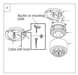
Hang motor assembly onto the buckle on mounting plate for hands-free wiring and safety cable installation.
