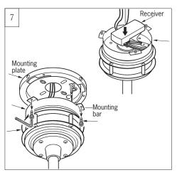
Place receiver in position as shown. Remove set screws from mounting bar with allen wrench provided.
