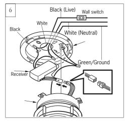
Make wiring connections using wire connectors provided as indicated above. White from house to White from remote receiver marked AC IN N. Black from house to Black from remote marked AC IN L. Connect all green grounded wires to Grounded wire from House. Make sure that no filaments are outside of the wire connector.
