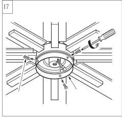
Remove 3 set screws from side of light pan. Keep screws
