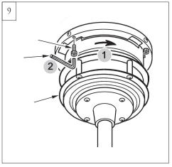
Align the holes on mounting plate with the screw holes in mounting bar. Reinstall the screws removed in step 7. Tighten all screws securely.
