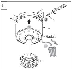
Lift fan housing up, aligning the holes on housing with the holes on mounting plate.
