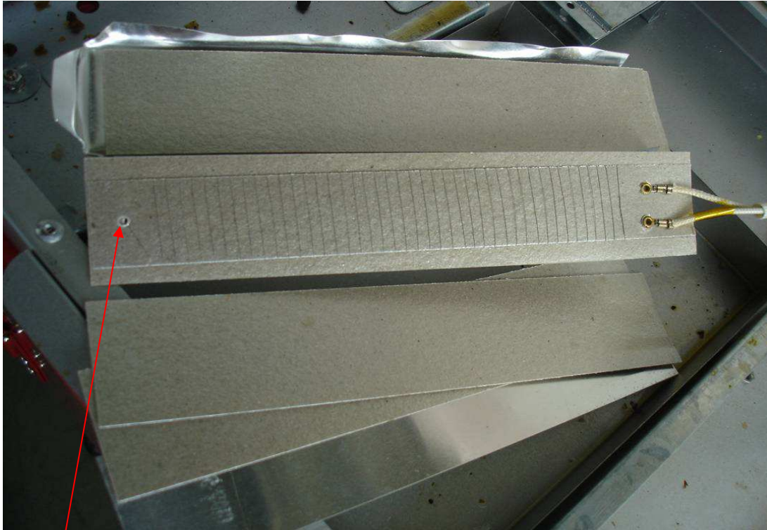
Fixed by riveting
