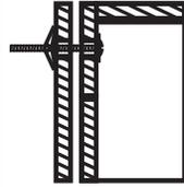
**DRYWALL:** Drill holes and secure to the wall with toggle bolts. Note: Use toggle bolts only when cabinet cannot be attached to a wall stud. Cabinet must also be attached to adjacent cabinet as outlined in Step 3.
