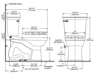
THIS TOILET IS DESIGNED TO ROUGH-IN AT A MINIMUM DIMENSION OF 305MM (12") FROM FINISHED WALL TO C/L OF OUTLET. SUPPLY NOT INCLUDED WITH FIXTURE AND MUST BE ORDERED
