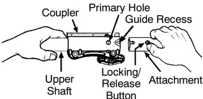
**WARNING:** Make sure the locking/release button is locked in the primary hole and the knob is securely tightened before operating the unit. All attachments are designed to be used in the primary hole unless otherwise stated in the applicable attachment instruction manual. Using the wrong hole could lead to serious injury or damage to the unit.
