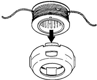
10. Insert the ends of the lines through exit holes in the sides of the cover.
