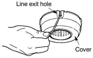
11. Reinstall the spool and cover onto the trimmer head. Push until cover snaps into place.
