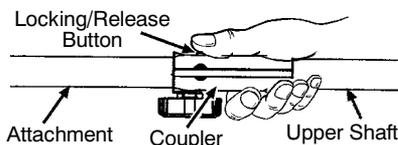
3. While securely holding the engine and upper shaft, pull the attachment straight out of the coupler.
