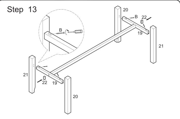
Attach crossbars (19) to legs (20,21) using screws (B). Attach end caps (22) to crossbars (19) using dowels as guides.
