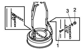
**4.** Attach the Post/Post Support Plate (F) to the Post Supports (H). Align the Post/Post Support Plate (F) with the holes in the tops of the Post Supports (H) and insert M6x20 Bolts through holes. Secure on the underside with M6 - Nuts. Hand tighten initially then tighten with a wrench when all bolts have been inserted. Slide the Tank Housing (E) over the Post and rest on the Base.
