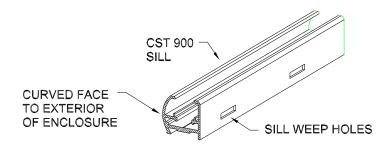
2. Position Sill (B) on center of curb. Using the Sill's pre-drilled holes as guides, mark and drill three 1-1/2'' deep installation holes using a 1/8'' drill bit. Insert three Plastic Screw Anchors (D) into installation holes, reposition Sill (B) and secure it to curb using three Installation Screws (E).
