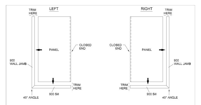
1. According with left / right selection, trim both CST 900 profiles 1/2" longer than Panel height and width.
