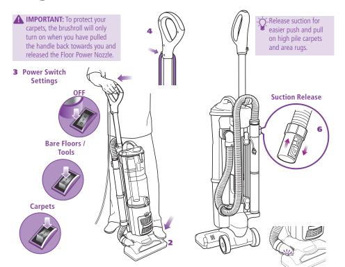
Your **Shark® Navigator™ DLX**Vacuum can be used to clean bare floors or carpets — with the click of a switch.
