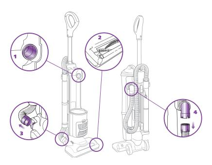
Unplug the vacuum before checking for blockages.
