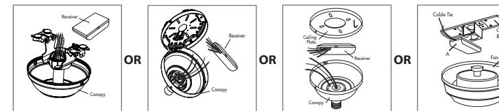
**Note:** Some fans may have considerable excess lead wire. For easier canopy installation, cut the excess wire, leaving a minimum of 8" remaining. Re-strip the fan lead wires 1/2". Place remaining excess wire into the ceiling electrical box. **The bracket and fan must remain properly grounded.**
