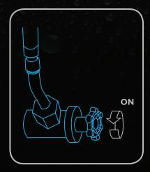
Turn your house's water back on. Make sure water isn't leaking anywhere. If it is, check the connections and tighten if necessary.
