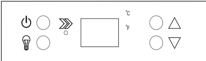
Indicator light illuminates to signify the cooling mode is currently in operation.
