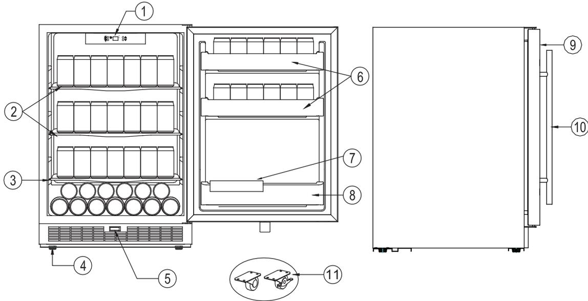
1. **Control panel** : For viewing and regulating the temperature for the refrigerator.
