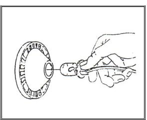
**CAUTION:** The replacement bulb must be the same rating as the factory installed bulb.
