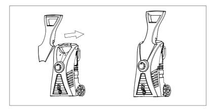
• Then using 4 screws provide and a screwdriver(no supplied), screw the handle to the power washer from back of machine.
