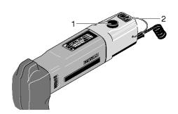
A material oriented speed/stroke can be adjusted by turning the control knob **1**. Use higher speeds for wood, aluminum, brass and circuit boards, lower speeds for plastics, specially thin materials and very delicate work pieces.
