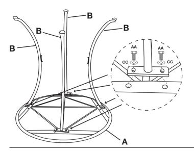
Attach the legs (B) to the table top (A) using bolts (AA) and washers (CC). Tighten using the wrench (EE).
