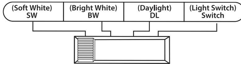
**NOTICE:** The toggle switch is located on the back of the fixture.
