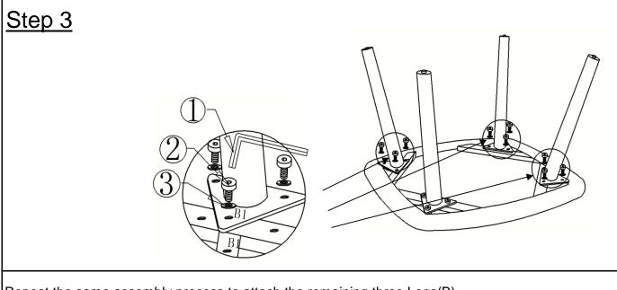
Repeat the same assembly process to attach the remaining three Legs(B). **Do not fully tighten the Bolts.**
