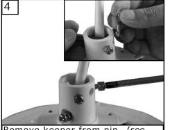
Remove keeper from pin. (see inset) Loosen the 2 set screws in yoke for downrod to slip into yoke.
