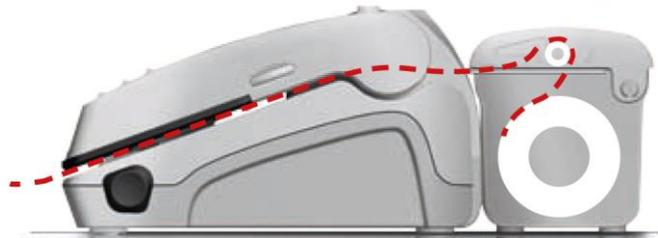
3. Open the top cover of the vacuum sealer and pull the desired length of bag through the slot in the top cover.
