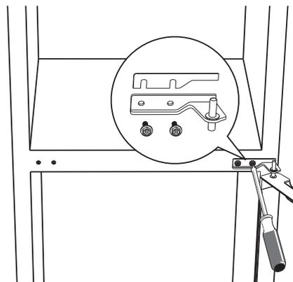
8. Move the hinge hole cover of lower door from left side to right side.
