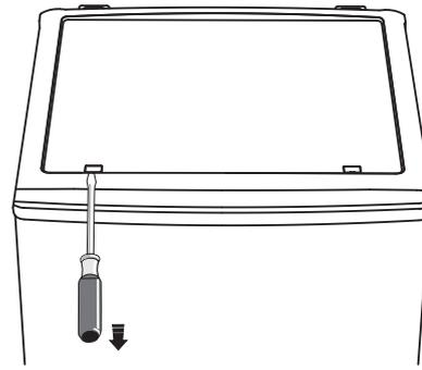
3. Remove the 2 screws on the back.
