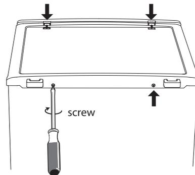
17. With the doors closed, check that the doors are aligned horizontally and vertically and that the seals are closed on all sides before finally tightening the bottom hinge. Re-adjust the levelling feet as needed.
