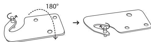
7. Take off the middle hinge by removing the screws. And then lift the lower door and place it on a padded surface to prevent it from scratching.
