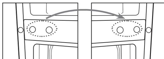
9. Remove the screws and bottom hinge. Then remove the adjustable feet from both side.
