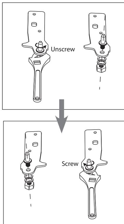
11. Refit the bracket fitting the bottom hinge pin. Replace both adjustable feet. Transfer the lower door to the property position.
