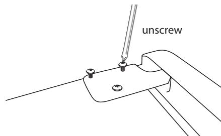
6. Remove the bolt with a screwdriver and flip the hinge bracket. Then reattach the bolt to the hinge bracket.
