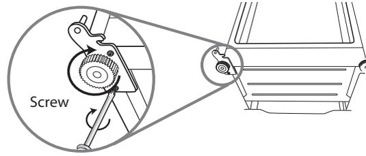
12. Make the middle hinge reverse the direction 180°C, then transfer it to the left property position. Make the middle hinge pin in the upper hole of the lower door, then tight the bolts.
