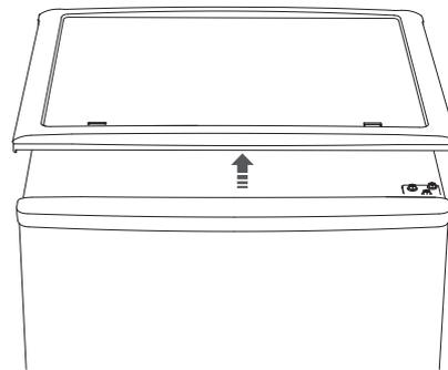
5. Remove the three screws, then remove the upper hinge that hold the door in place. Lift the door and place it on a padded surface to prevent it from scratching.
