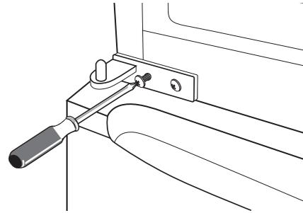
13. Place the upper door back on. Ensure the fridge door is aligned horizontally and vertically so that the seals are closed on all sides before finally tightening the top hinge.
