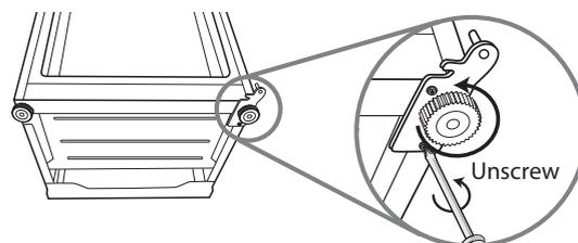
10. Unscrew and remove the bottom hinge pin, turn the bracket over and replace it.
