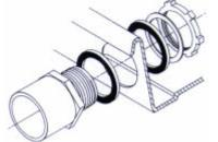
Drill 1-3/8" dia. hole on side or bottom surface of DURAPAN<sup>™</sup> and install fitting as shown. Position DURAPAN<sup>™</sup> and connect solventweld fitting to 1" PVC pipe (not provided) leading to drain pipe. Place wash machine inside DURAPAN<sup>™</sup> to complete installation. Contents: Washing machine pan and 1" PVC drain fitting.
