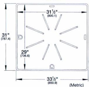
General: Furnish and install as shown on plans, DURAPAN<sup>™</sup> Wash Machine Pan model 96, as manufactured by E.L. Mustee & Sons, Inc. One-piece compression molded Co-PolyPure<sup>™</sup>, using matched metal molds. Shall include (1) 1" PVC fitting. Color:White Install in compliance with local codes.
