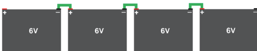
Figure 9.5 Four 6V batteries connected in series
