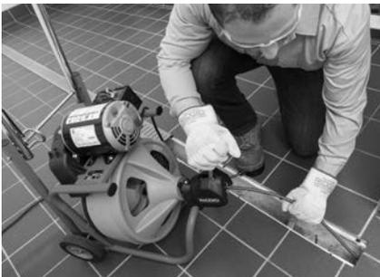
**Figure 15 – Operating K-400 with AUTOFEED**
