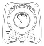
a. **DISC**— Rotate the control clockwise away from ALL METAL to get DISC mode. The DISC mode comes with auto ground balance. Rotate the control slowly and clockwise to eliminate different trash objects.
