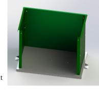
gently lift the rear panel vertical so that the larger tabs on each end of the rear panel engage with the slots cut into the upright corners of the side panels. Once the Rear Panel is engaged with the sides on each end, place a 1/4" x 3/4" carriage bolt (from the outside) into the square holes half way up the side panels. Place a 1/4" nut and 1/4" flat washer on each bolt, and tighten.
