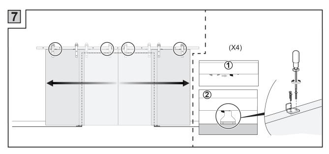
Set the catches on the soft-closing mechanism to the open position. To determine the positioning of the soft-close triggers, it is recommended that the doors be moved to the fully open position. Determine where the soft-close trigger would engage the soft-close mechanism and mark your drill holes on the top of the door. Move the door to the fully closed position and repeat to determine the placement of the second soft-close trigger.
