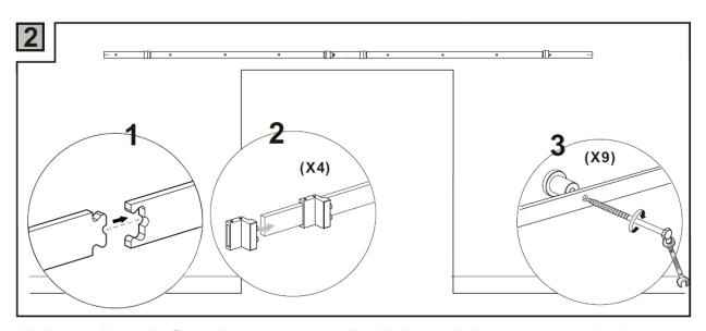
Join the two rails together. Fasten the door stops to the rail at this time, two in the center, two at each end. Attach the rail to the wall brackets using a wrench to fasten the bolts.
