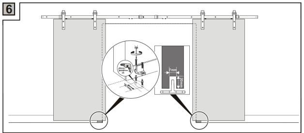
Plumb the door and mark the positions of the floor guides. Mount the floor guides to the floor.
