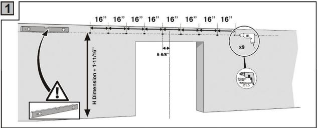
Find the centerline of the track. Using a level, mark a horizontal line twice the door width long. Mark the bracket screw locations into the wall blocking. Attach the wall portion of the brackets as shown.
