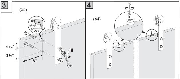
Drill out holes in the door using a 10mm routing drill bit as pictured. The bottom of the doors should be routed at this time in order to accept the floor guide.
